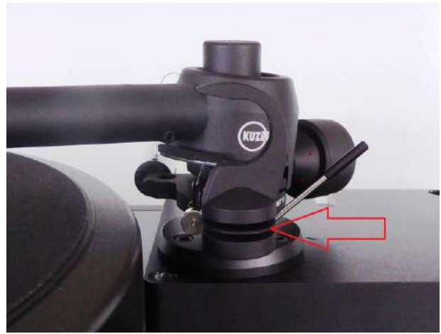
Fig. 13a. Arm rest one spacer plate
