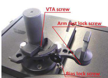
Fig. 5. Arm tower- various adjustments
