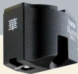
Hana S Series MK II cartridges use a new tapered aluminum cantilever with higher rigidity, and effective mass reduction at stylus tip, resulting in enhanced clarity and music transfer from vinyl record to cartridge generator.
